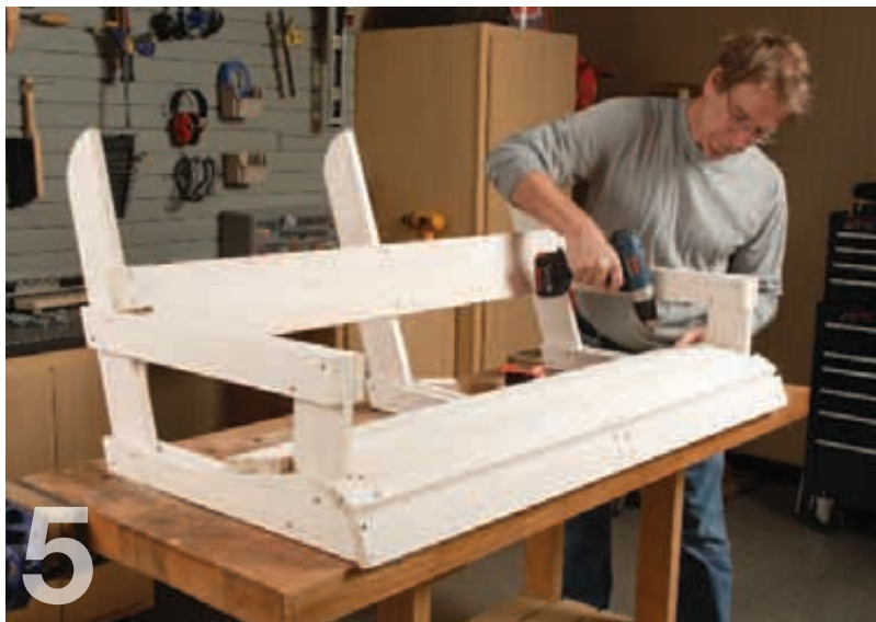
5 Space the outer frames 4 ft. apart and center the middle frame. Install the first seat slat and the lowest back slat to hold the frames square; then install the remaining slats. Drill a 1/8-in.-dia. pilot hole for each screw.
